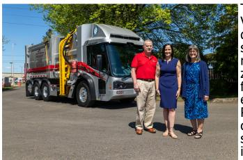
The two McNeilus Volterra ZSL trucks were designed to meet stringent environmental regulations and hold a zero-emission certificate from the US environmental Protection Agency. They come with extensive safety features including: a 360-degree camera system, blind-
